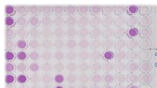
Figure 4. Schematic representation of the microtiter plate-based assay for selecting lipases. This method is the benchmark method to select lipases most relevant for detergent and textile sectors.
