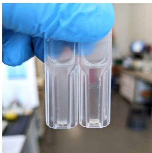
Figure 1: Turbidity assay, blank cuvette with sample treated with water and cuvette with sample treated with BCS366 culture supernatant.
