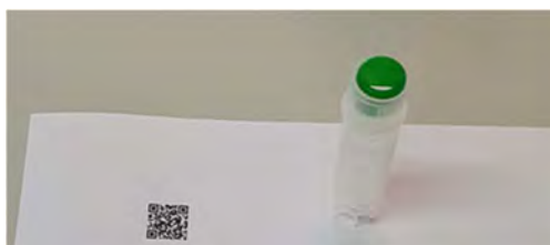
Image 1. Example of QR-coding a 2 mL tube. The size for the QR code to be printed is 0.8 x 0.8 cm. If the top of the lid is hollow, a lid filler can be placed to have a flat surface (a green lid filler is shown in the picture).
